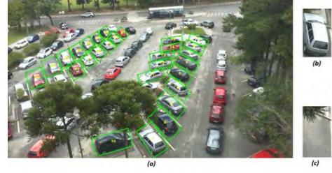
Figure 2. Segmented image: (a) 28 delimited spaces, (b) occupied sub-image, and (c) empty sub-image.
